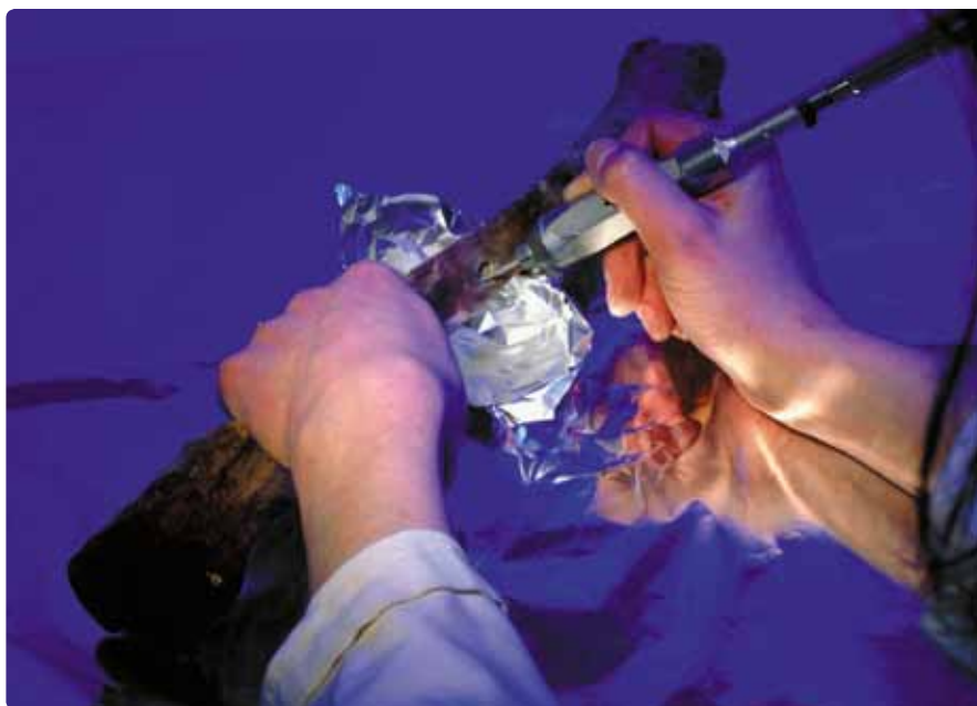
Sample being removed from bone for carbon dating using accelerator mass spectrometry (AMS). The bone is a human femur that is thought to date to the Middle Ages.
