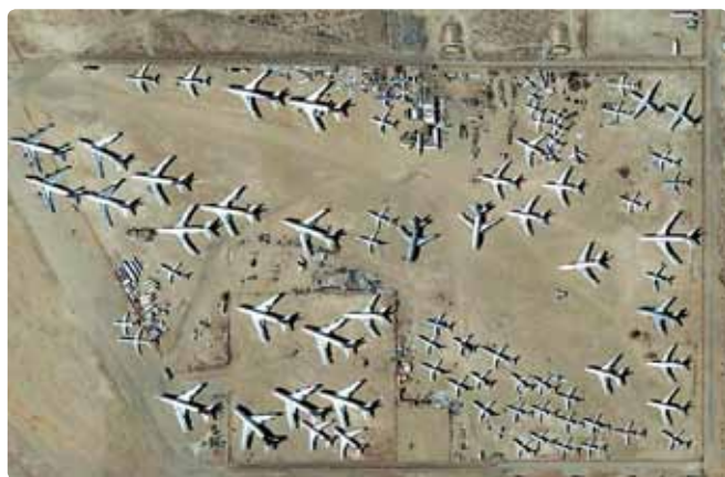
The planes in the Mojave Desert 'boneyard' are preserved from rusting by the dry desert air and low rainfall.
