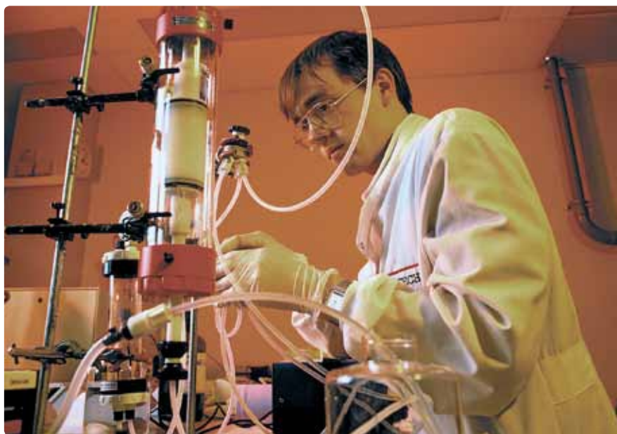
A chromatograph automatically separates mixtures by chromatography.
