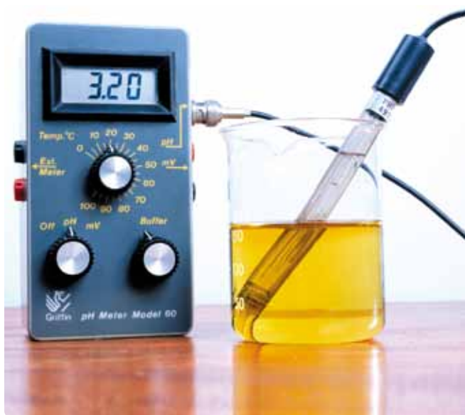
A pH meter measures the number of hydrogen ions that are in the liquid and uses this to calculate the pH which is displayed on the screen.
