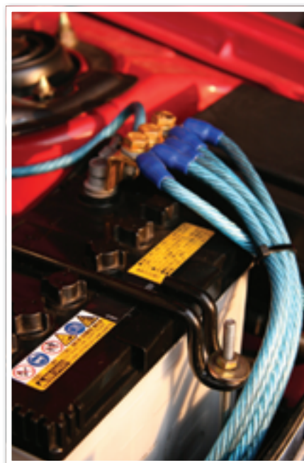
Fig 7.2.7 A car battery uses a series of wet cells to generate its 12 volts.
