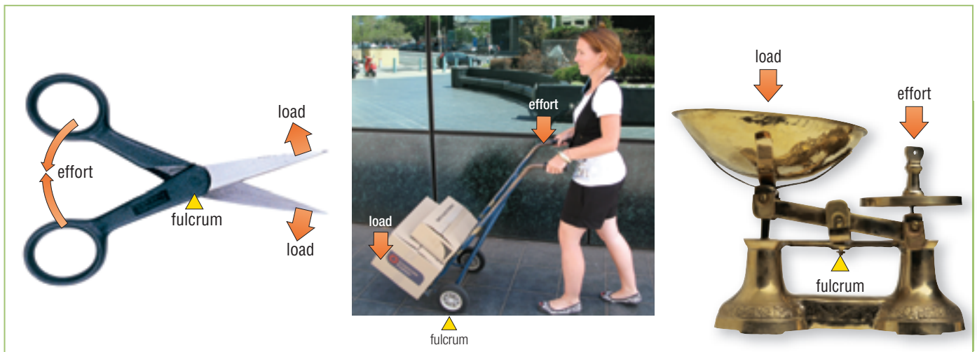
Fig 8.2.4 Class 1 levers resemble a seesaw, the fulcrum being somewhere in the middle of the lever.
