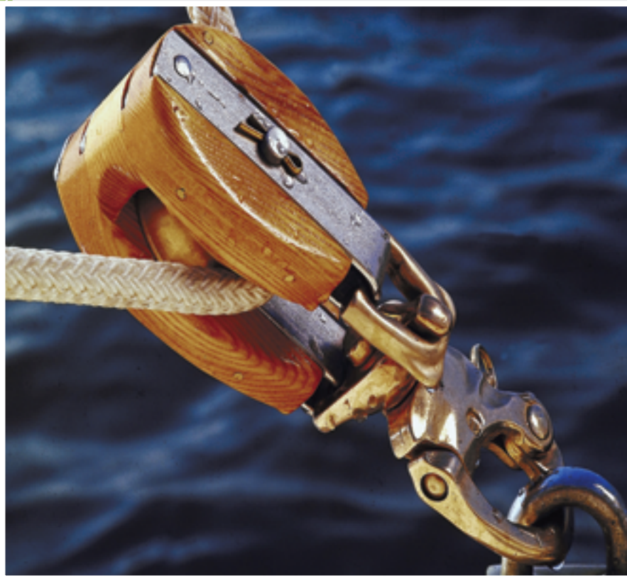
Fig 8.4.1 A pulley is a wheel with a grooved edge inside which a string, rope or chain can run.
