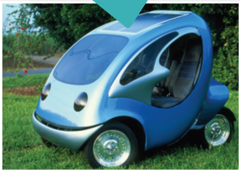
Fig 7.2.9 Sunlight falling on a photovoltaic cell forces electrons from one layer to the other, causing an electric current. This solar-powered car has a solar panel made from photovoltaic cells on its roof.
