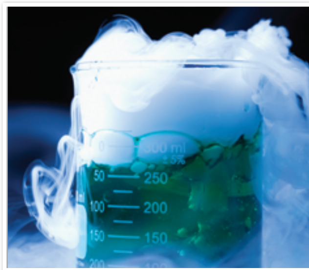
Fig 2.2.2 Frozen carbon dioxide in water undergoes a physical change from solid to gas.
