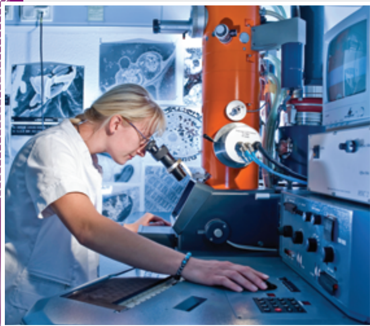
Fig 5.1.5 A microbiologist using an electron microscope. Only electron microscopes are powerful enough to make viruses visible.
