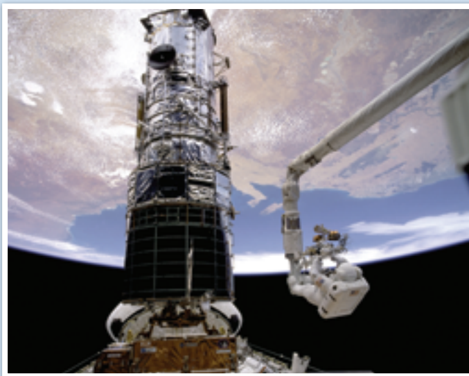
Fig 9.3.7 Astronauts carry out mirror repairs on the Hubble Space Telescope (HST) from the space shuttle Endeavor .
