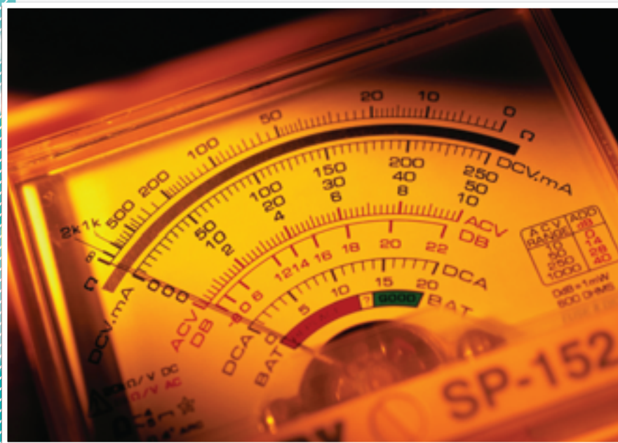
Fig 7.2.1 Current electricity is moving electricity. An ammeter measures how much current is flowing through it, whereas a voltmeter measures the energy used as the charges move through a component in the circuit.
