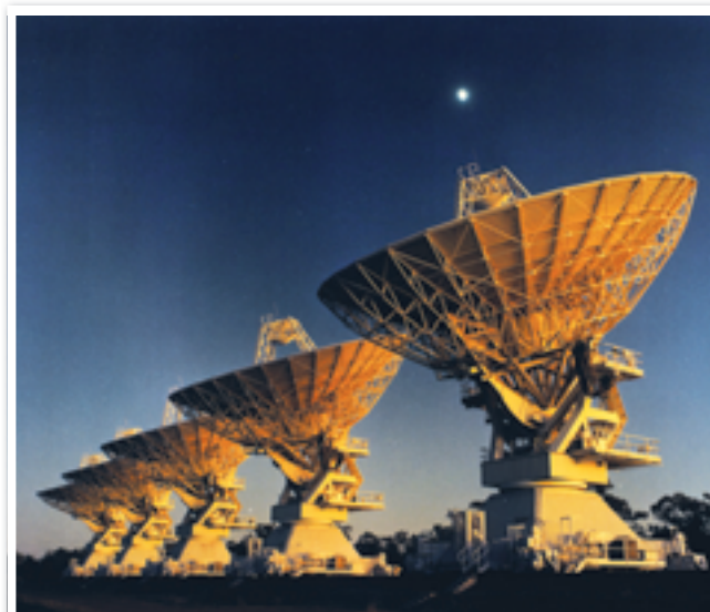
Fig 9.3.6 The Australian telescope compact array near Narrabri in New South Wales detects radio waves from objects such as pulsars. Several telescopes are placed together so that they form the equivalent of a much larger single telescope.
