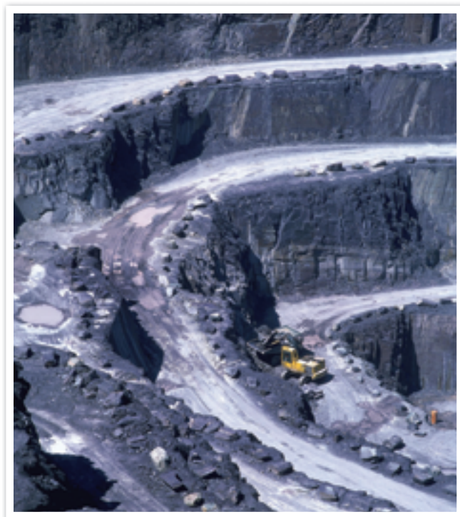
Fig 2.2.7 An open-cut mine showing benches
