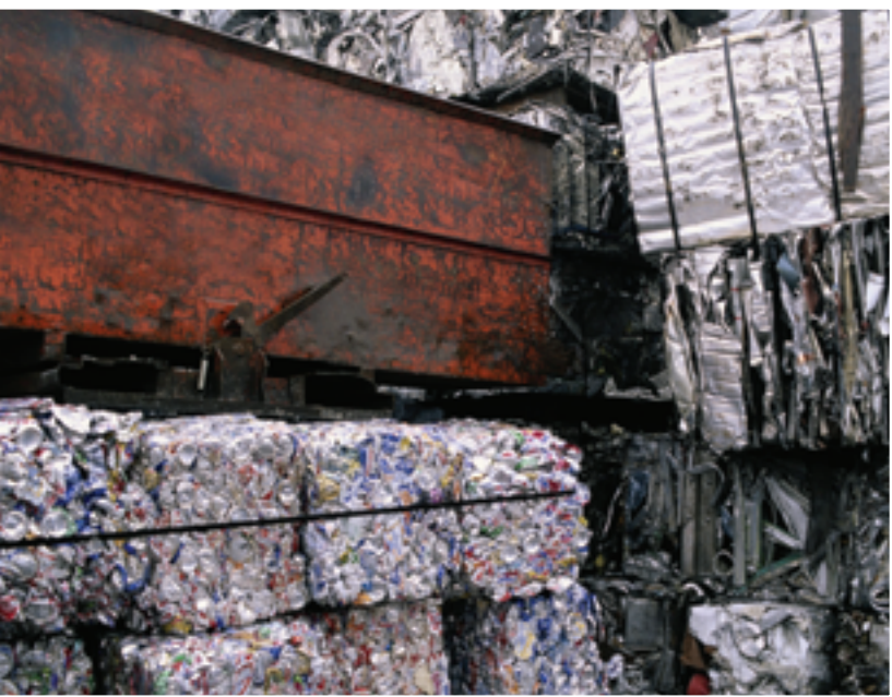
Fig 2.2.11 It is cheaper to recycle than to produce new aluminium. For this reason, more than 50 per cent of all aluminium cans in Australia are collected and reprocessed.
