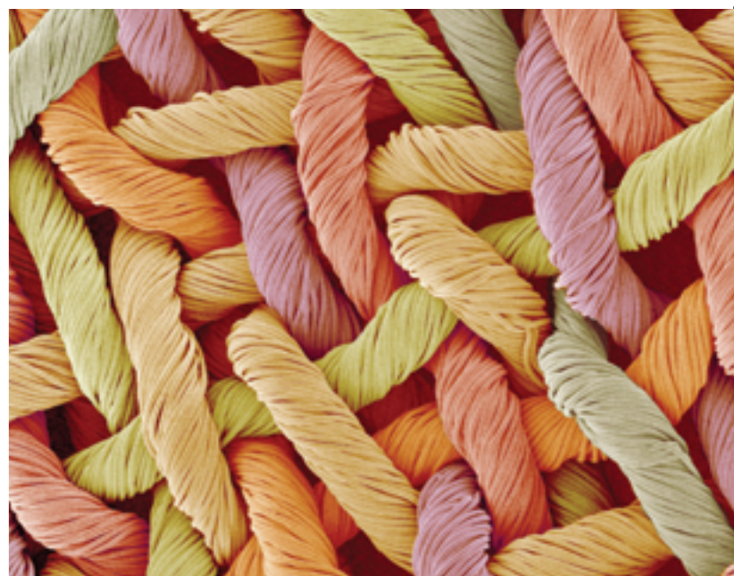
Fig 2.4.1 Fibres are the strands that are woven together to make fabrics. This scanning electron microscope (SEM) image is of georgette crepe, a fabric woven from synthetic fibres.
