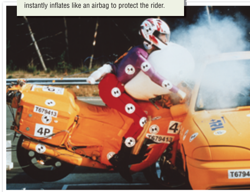
Fig 6.3.6 Although inflatable airbags have been tested on motorbikes, inflatable jackets have been developed to protect riders in case of an accident.
