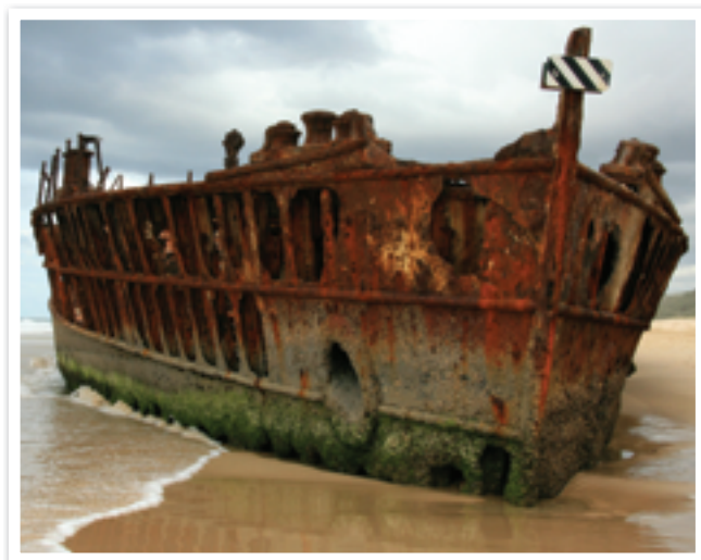
Fig 1.2.5 Rusting is a slow reaction but one that eventually destroys unprotected iron and steel in bridges, buildings, cars, machinery, and in this case, ships. Rusting is an example of an oxidation reaction.
