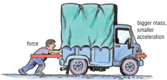
Fig 6.4.2 Acceleration depends on mass and the force applied.
