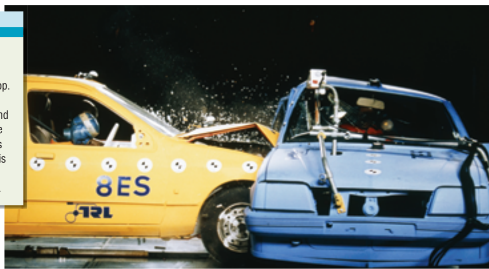
Fig 6.4.3 Crumple zones increase the time over which an accident happens. They decrease deceleration and decrease the impact forces on the occupants. All this technology is useless, however, if seatbelts are not worn.
