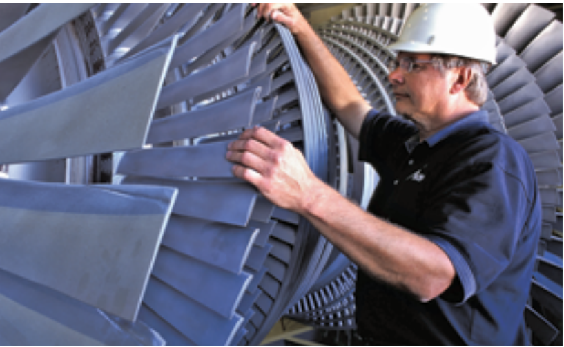
Fig 7.2.13 Compare the size of the person in this photo with the steam-driven turbine used to generate electricity.
