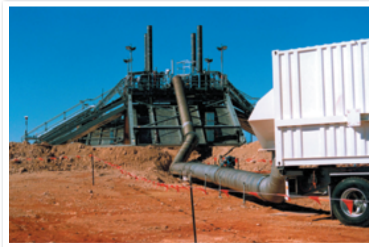
Fig 8.3.10 Four giant electrodes can be seen at the top of the in-situ vitrification equipment. The large pipe connected to the truck channels exhaust gases from the melt for analysis.
