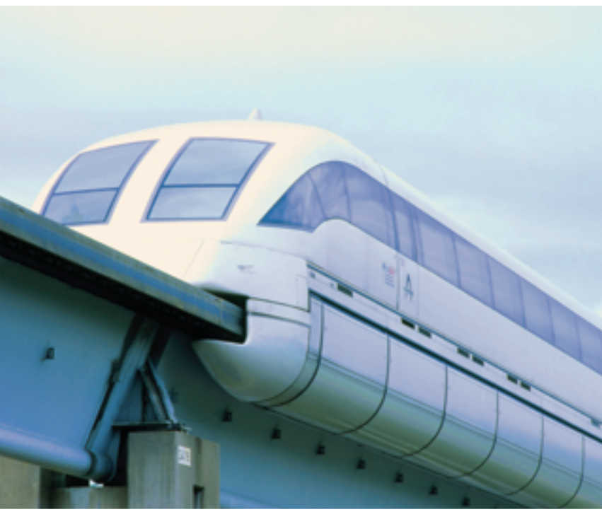
Fig 7.2.1 A Maglev train on trial in Germany. Maglev trains use electromagnetism to repel themselves off the track so that they float above it. Electromagnetism also moves the train forward. Other Maglev trains are currently being tested in Japan.
