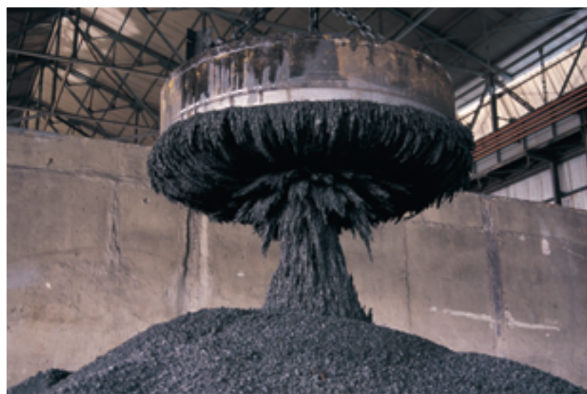
Fig 7.2.5 Electromagnets can be turned on and off and are generally stronger than permanent magnets. This makes them very useful in industry and in everyday electrical appliances.
