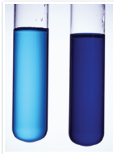
Fig 1.1.14 Concentrated solutions contain more of the chemical than a dilute solution. If coloured, a concentrated solution will be brighter or darker than a dilute solution.
