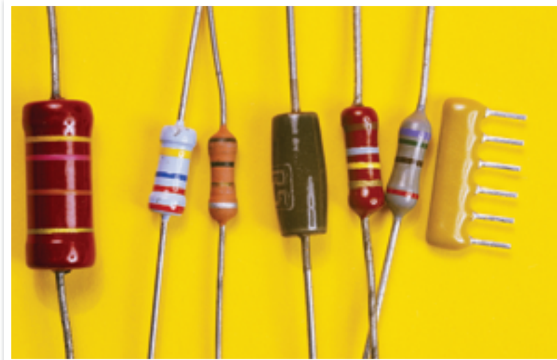
Fig 7.1.4 Resistors restrict the flow of current. Variable resistors are commonly used as volume controls on radios, MP3 players, TVs and sound systems.
