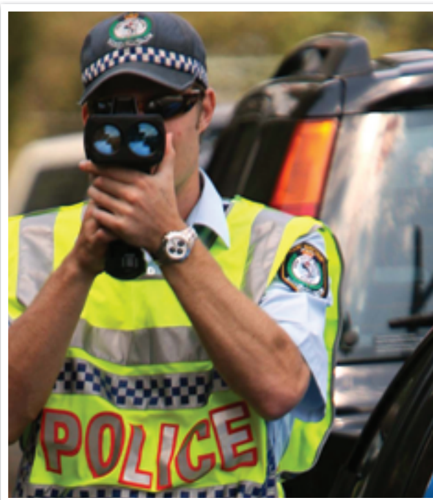
Fig 6.1.3 Police radar guns measure instantaneous speed.
