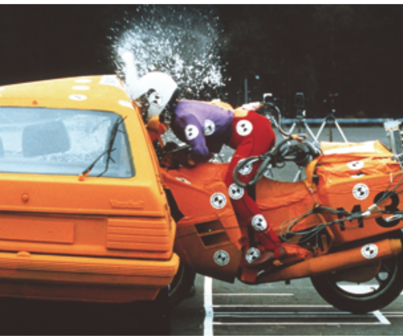
Fig 6.3.1 In this collision the rider has kept moving forward at the speed at which the bike was moving just before the accident. This is the effect of inertia. The rider will only stop when they hit something.
