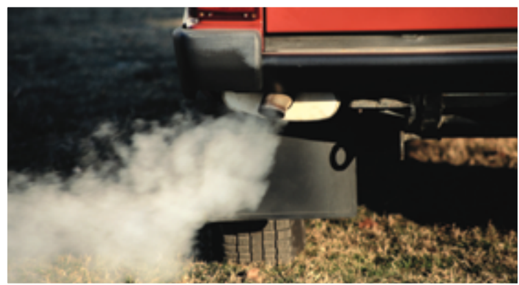
Fig 1.2.4 Incomplete combustion in car engines produces carbon, carbon monoxide and other chemicals that contribute to photochemical smog and air pollution.
