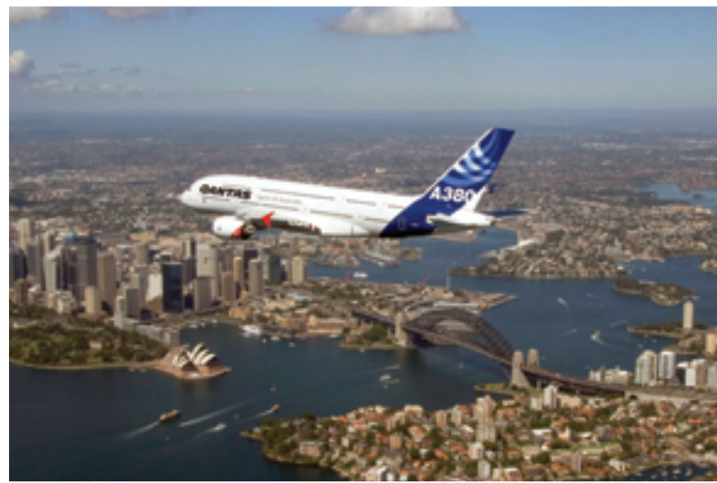
Fig 2.3.4 The Airbus 380 is the largest passenger aircraft ever produced, carrying up to 555 people over two decks. Roughly 22 per cent of the aircraft is made from an advanced lightweight plastic-composite material called CFRP.
