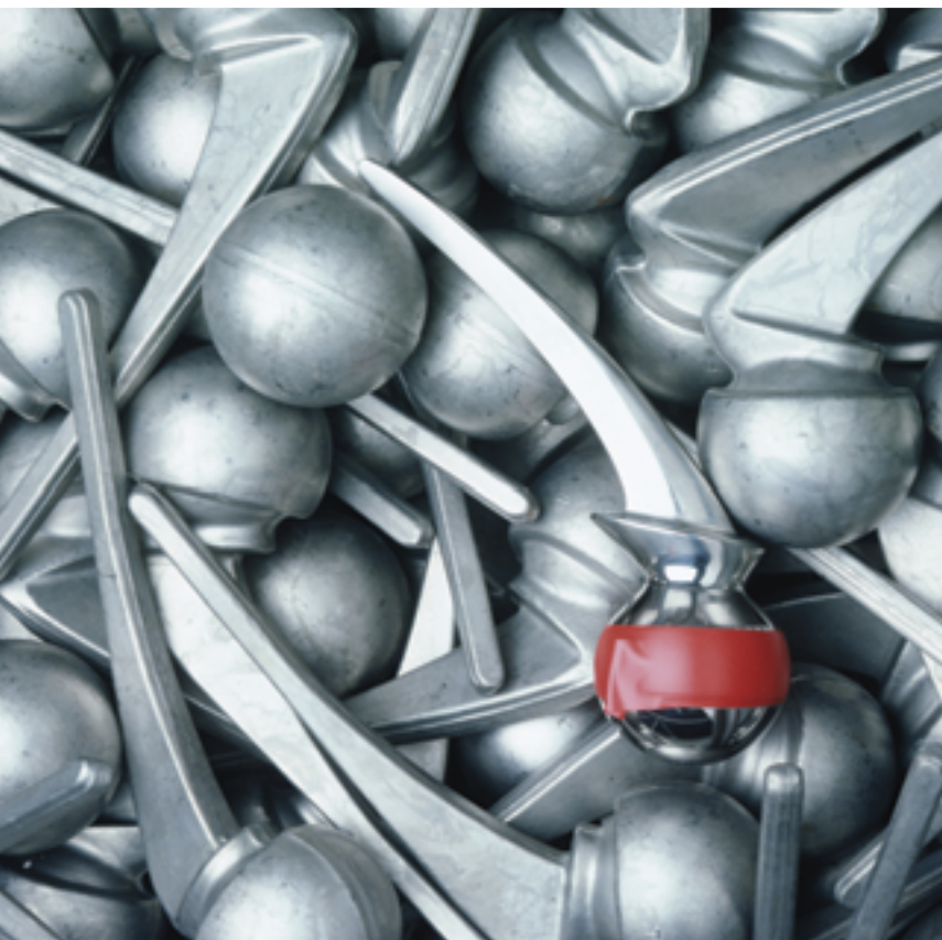
Fig 2.1.1 Artificial hip joints need to be strong, non-toxic, corrosion-resistant and made from a material that is unlikely to be rejected by the body. For this reason they are made from metal alloys of titanium, cobalt or chrome.
